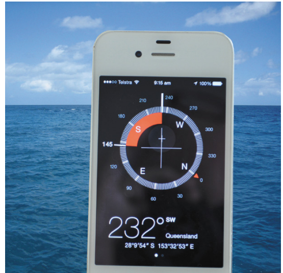
Figure 52.1 Magnetic bearing on a mobile phone app Wet Paper
