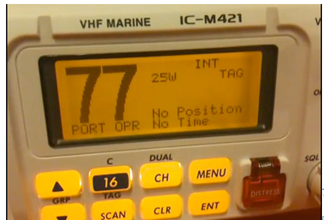
Figure 14.2 VHF radio with DSC - watch the video link
