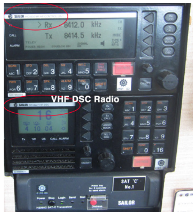
Figure 14.3 Ship VHF and MF/HF radios with DSC alert Wet Paper
